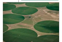
IRRIGATION This irrigation project in Colorado enables farmers to raise crops in the desert. Water from deep wells is pumped to sprinklers that rotate, forming circular patterns. Table of Contents
