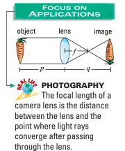
where p is the distance between an object being photographed and the lens and q is the distance between the lens and the film. Simplify the complex fraction.
